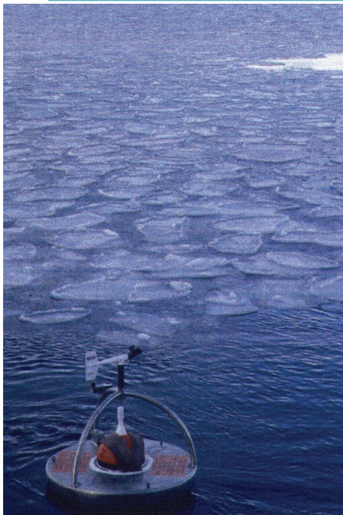
Drifter buoy measuring the deformation of the young pancake ice and its response to wind and wave action in the Weddell Sea, Antarctica. © Oli Peppe, DML.
